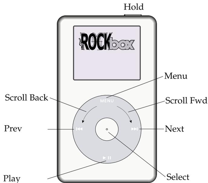
Throughout this manual, the buttons on the player are labelled according to the picture above. Whenever a button name is prefixed by “Long”, a long press of approximately one second should be performed on that button. The buttons are described in detail in the following paragraph. Additional information for blind users is available on the Rockbox website at [BlindFAQ](#). ▶
